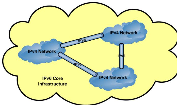
Figure 6: IPv6 Tunnelling with islands of IPv4 in and IPv6 core network (phase 2)
