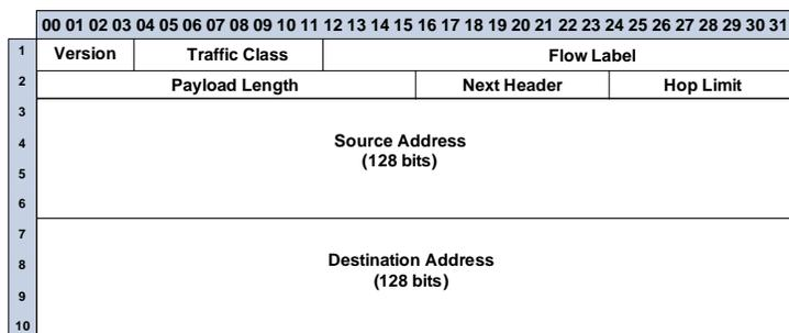
**Figure 3: IPv6 Structure**
