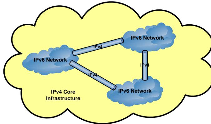
Figure 5: IPv4 Tunnelling with islands of IPv6 in and IPv4 core network (phase 1)
