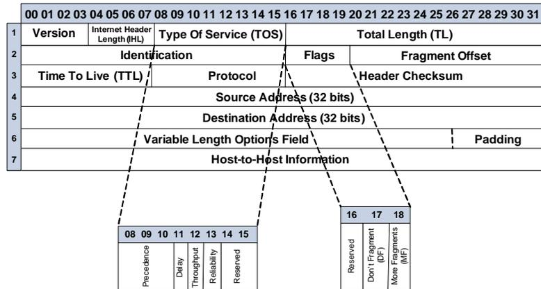
**Figure 2: IPv4 Structure**
