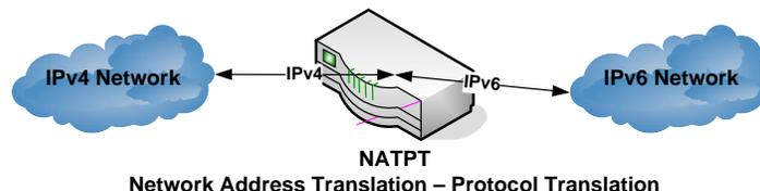
**Figure 7: The arrangement with Network Address Translation – Protocol Translation**
