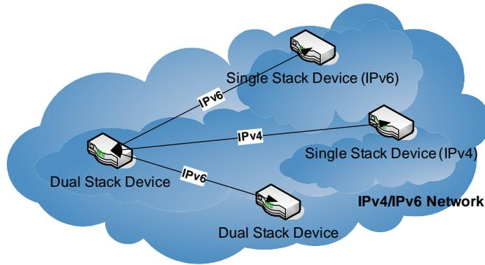
Figure 4: Dual stack operation
