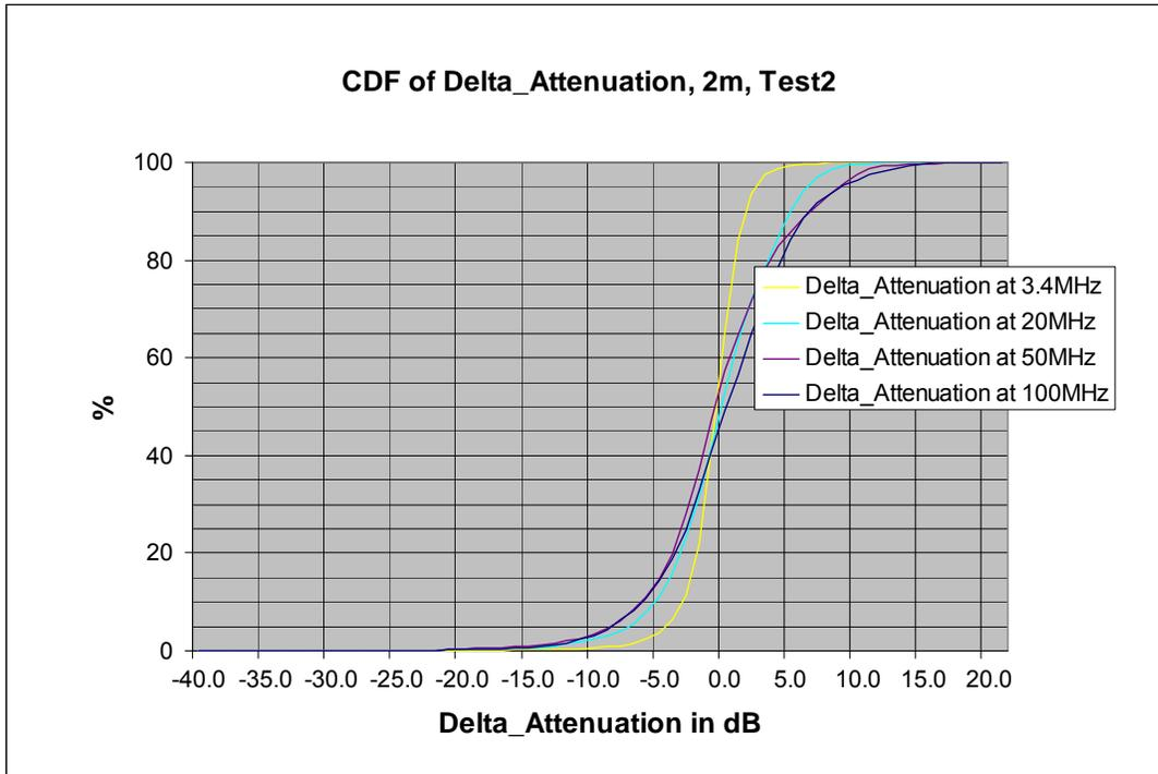
Figure 10: Example of measured CDF of path loss differences for different frequency offsets, 2m distance
