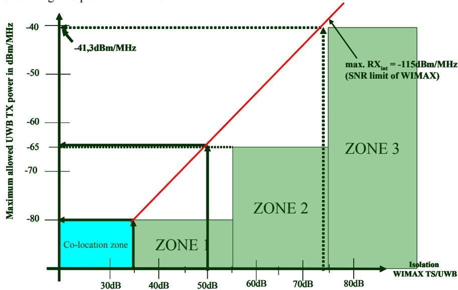
**Figure 7: Maximum UWB Tx Power at Downlink AMC Cell Edge**
