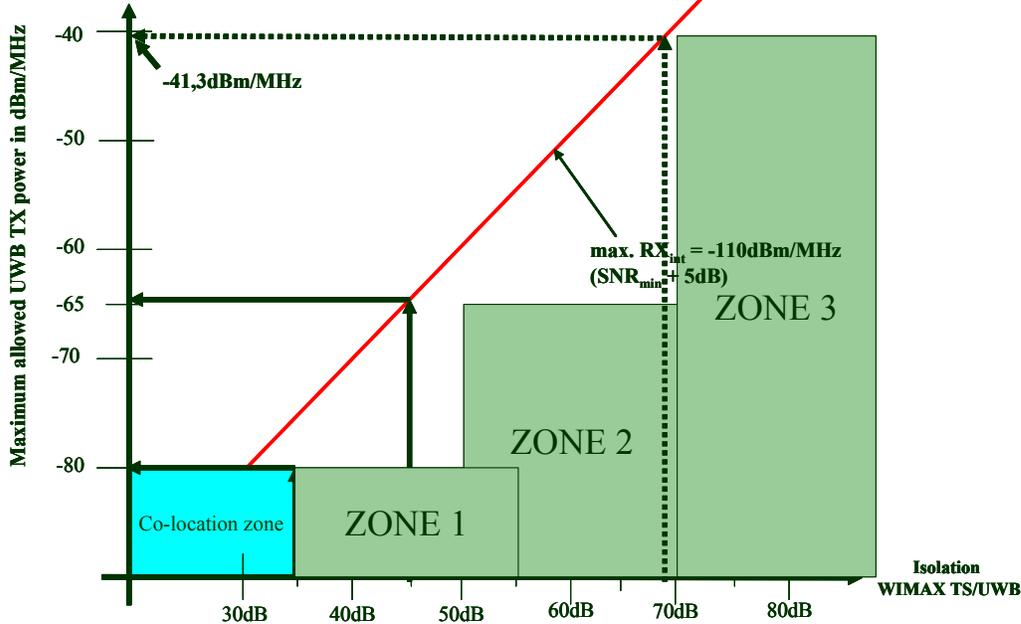
Figure 8: Maximum UWB Tx Power at Downlink AMC Inside Cell
