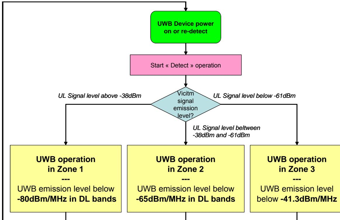
Figure 2: DAA flow chart revision in the frequency band 3.4-4.2 GHz
