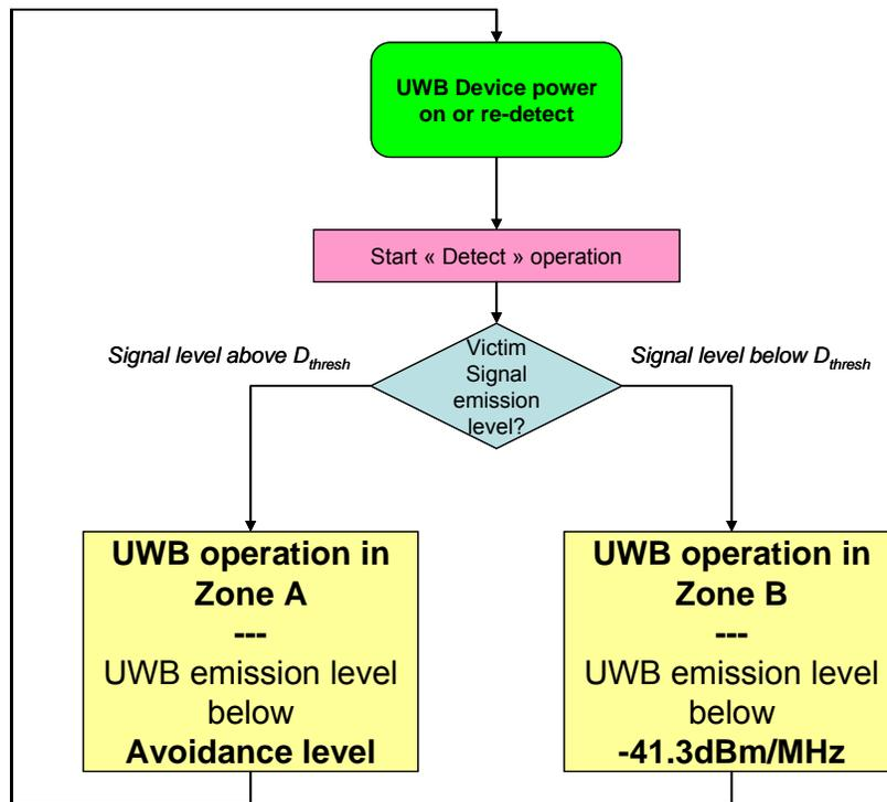
**Figure 1: DAA flow chart revision for radiolocation systems**
