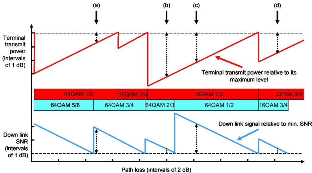
**Figure 9:** This figure shows how the BWA terminal transmit power will adjust downwards (relative to its maximum transmit power) and how the SNR on the downlink changes (relative to the minimum SNR for each modulation scheme) as the path loss is reduced. At points (b) and (d) the reduction in transmit power is greater than the margin above the minimum SNR. At point (c) the two are equal, and point (a) shows an example in which the SNR margin exceeds the reduction in transmit power
