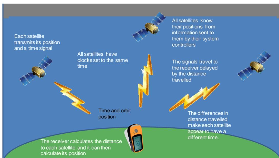
**Figure 2: RNSS/GNSS functionality**
