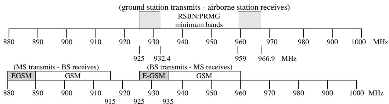
**Figure 2. Comparison of essential minimum spectrum requirements for GSM and RSN systems**
