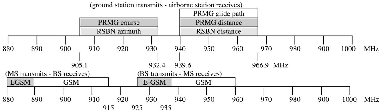
**Figure 1. Comparison of overlapping GSM and RSBN frequency bands**
