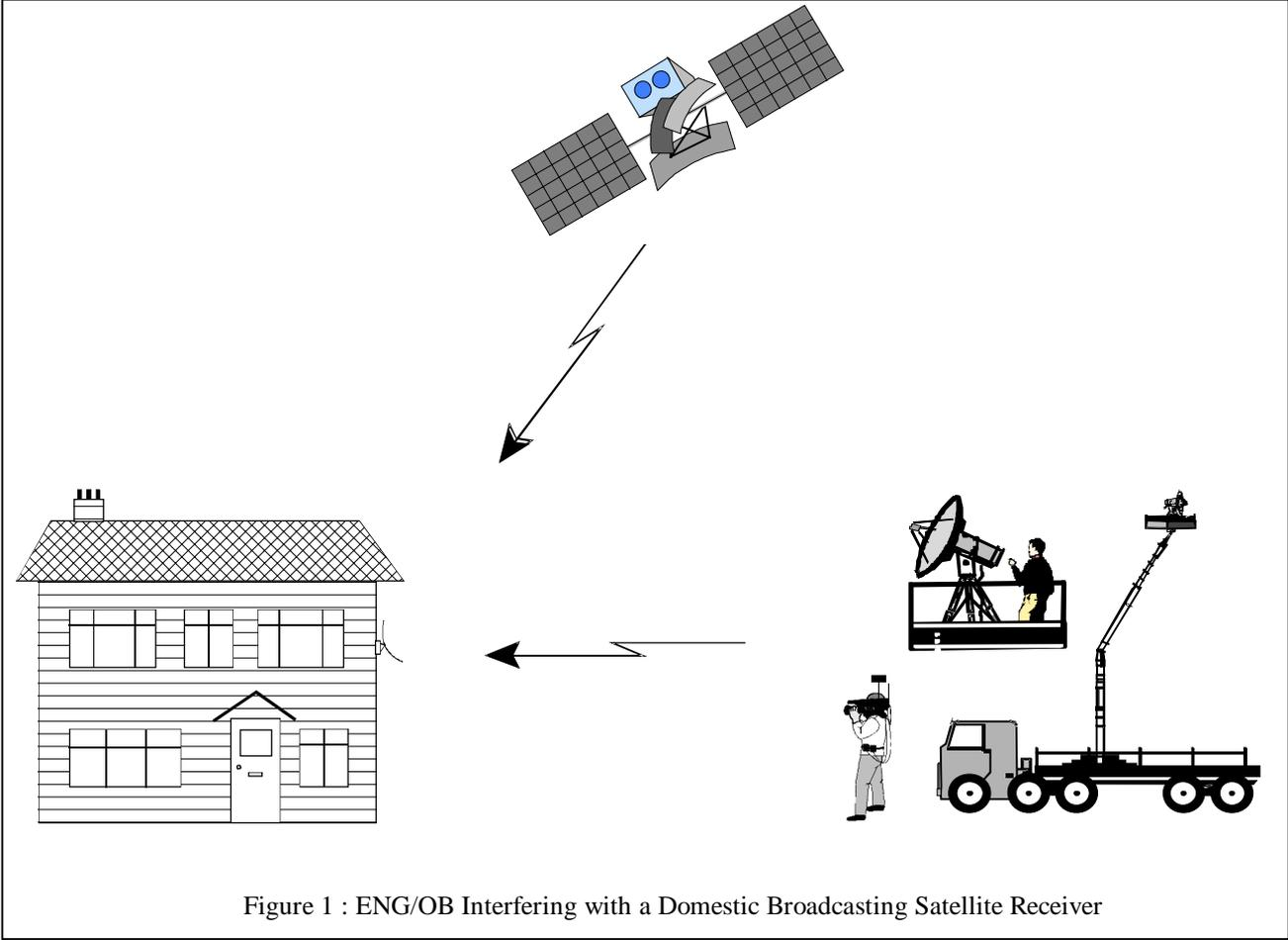
Figure 1 : ENG/OB Interfering with a Domestic Broadcasting Satellite Receiver
