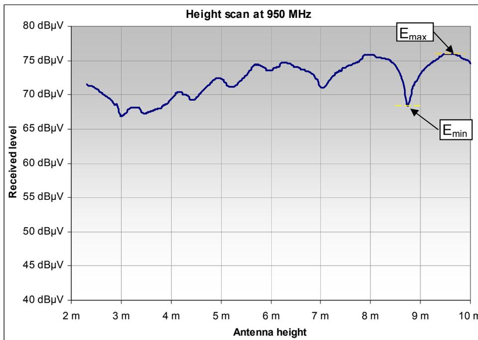
**Figure 1: Example of the dependency of the measured field strength on measurement antenna height**
