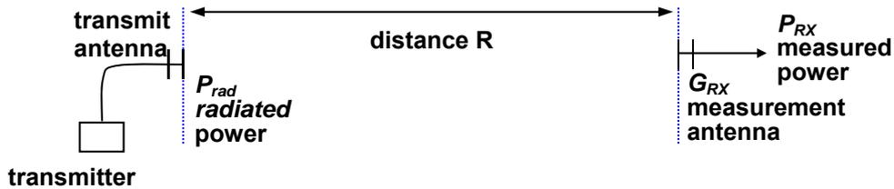
**Figure 5: radiated power measurement**
