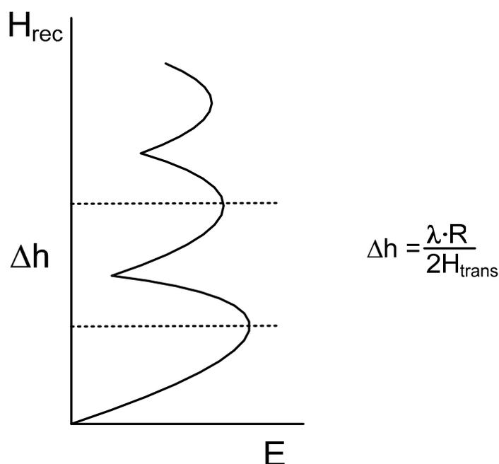
**Figure 4: The change of the field strength at change of height of the receiving antenna**
