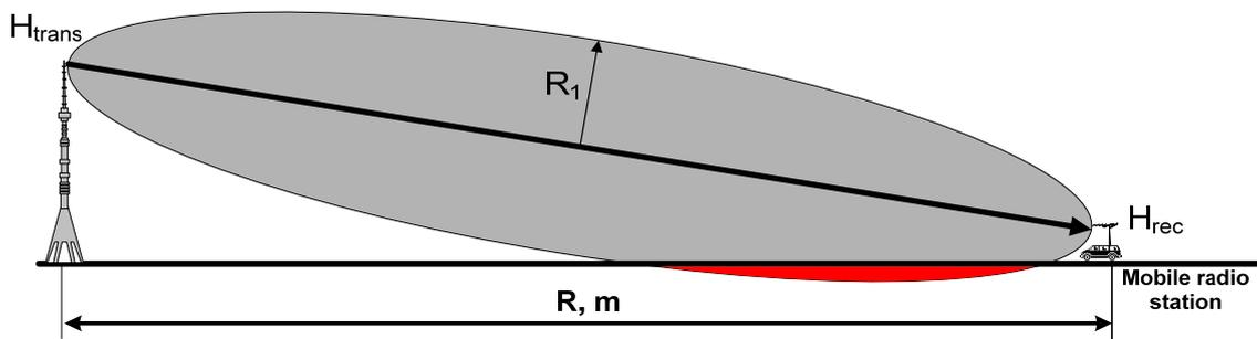
**Figure 3: The first Fresnel zone and the effect of the Earth's surface to the direct ray**
