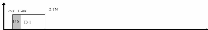
**VDSL1:** Up to 50 Mb/s, less than 1.2 km loop reach
