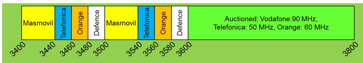
**Figure 14: Layout of 3400-3800 MHz band in Spain**
