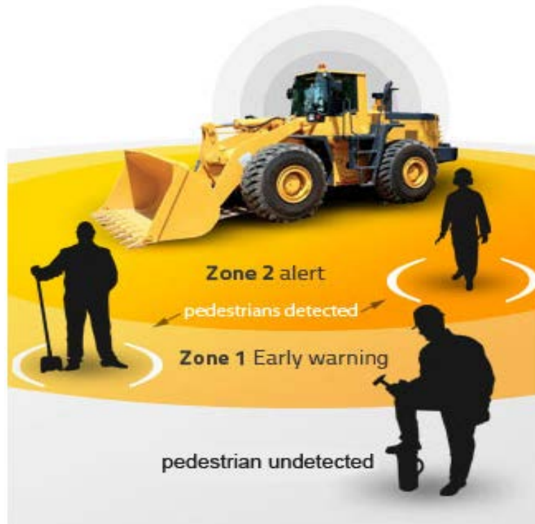
Figure 1: Detection and Collision Avoidance Principle
