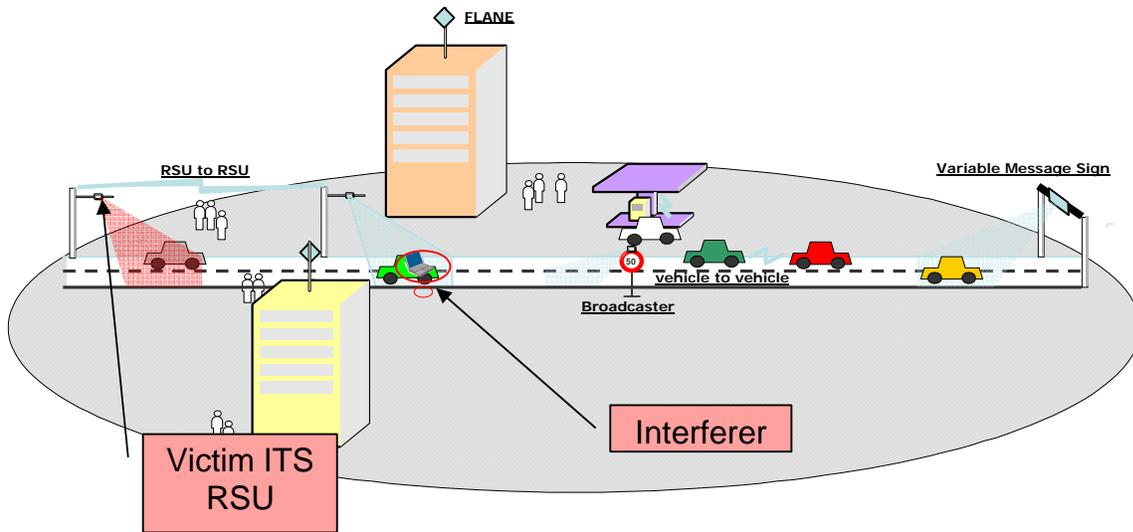
**Figure 10: Scenario 5 – ITS RSU possibly interfered with by MGWS-WLAN/WPAN located within a car**
