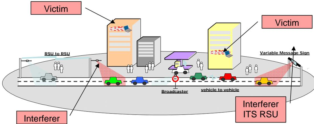
**Figure 7: Scenario 2 – MGWS-WLAN/WPAN possibly interfered with by a ITS RSU**
