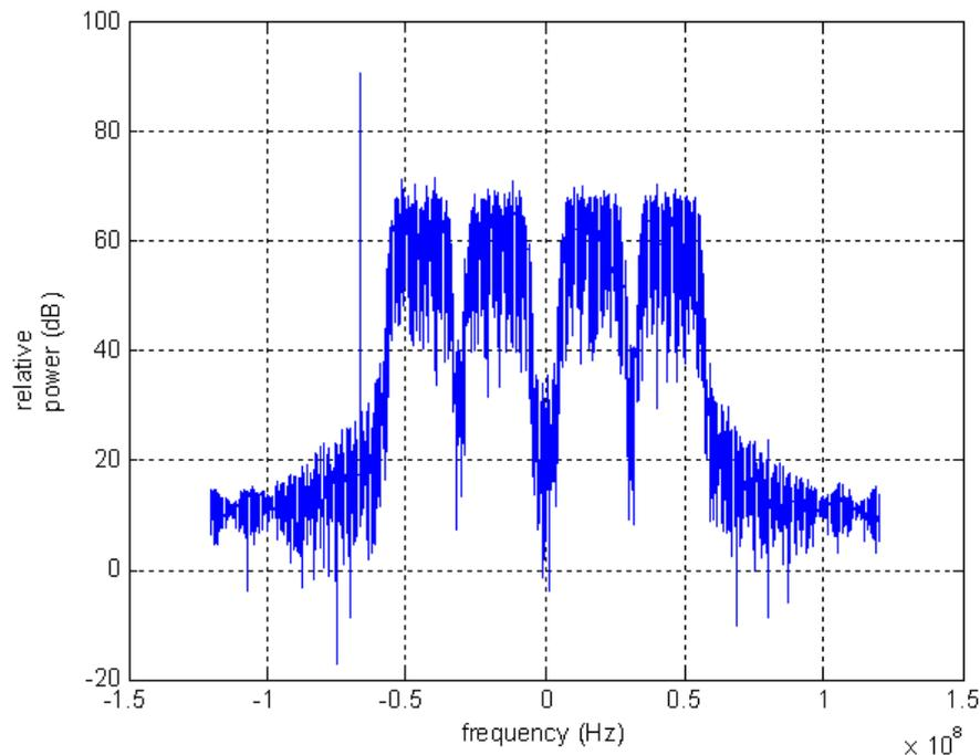
**Figure B.1: Baseband power spectrum of an RF ITS channel**
