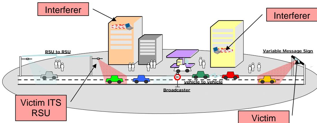
Figure 9: Scenario 4 – ITS RSU possibly interfered with by MGWS-WLAN/WPAN
