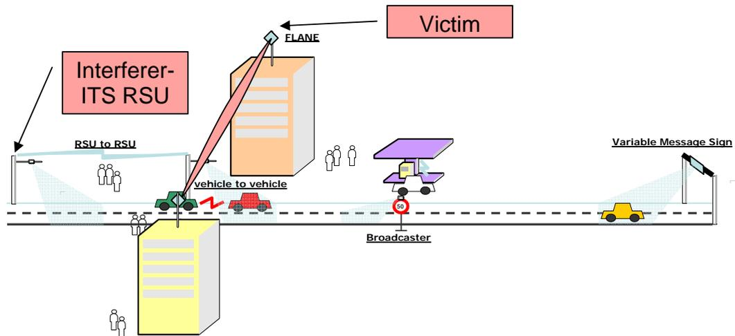
**Figure 5: Scenario 1-a – MGWS-FLANE possibly interfered with by an ITS RSU**
