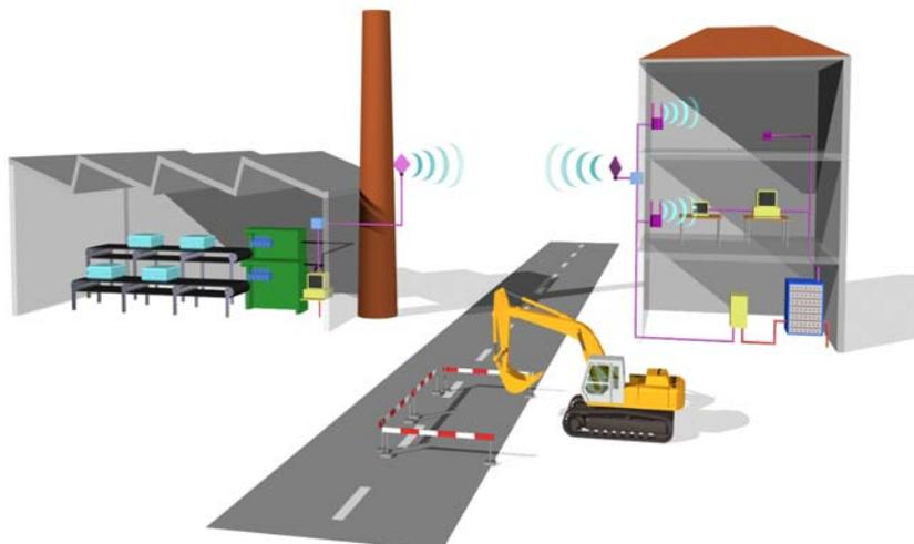
**Figure 4: Building to Building / FLANE LAN outdoor extension**
