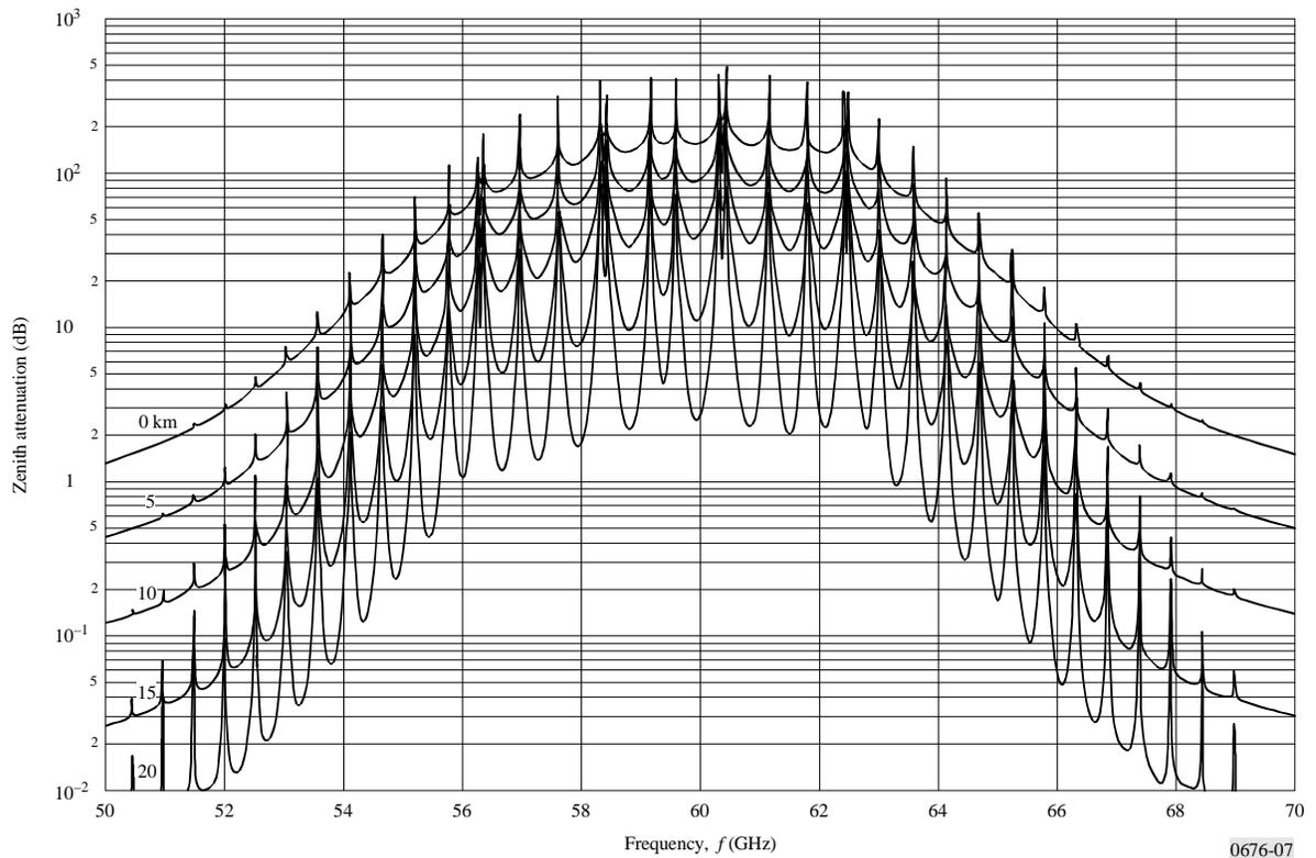
Figure A.2: Zenith Oxygen Attenuation (dB) – Recommendation ITU-R P.676
