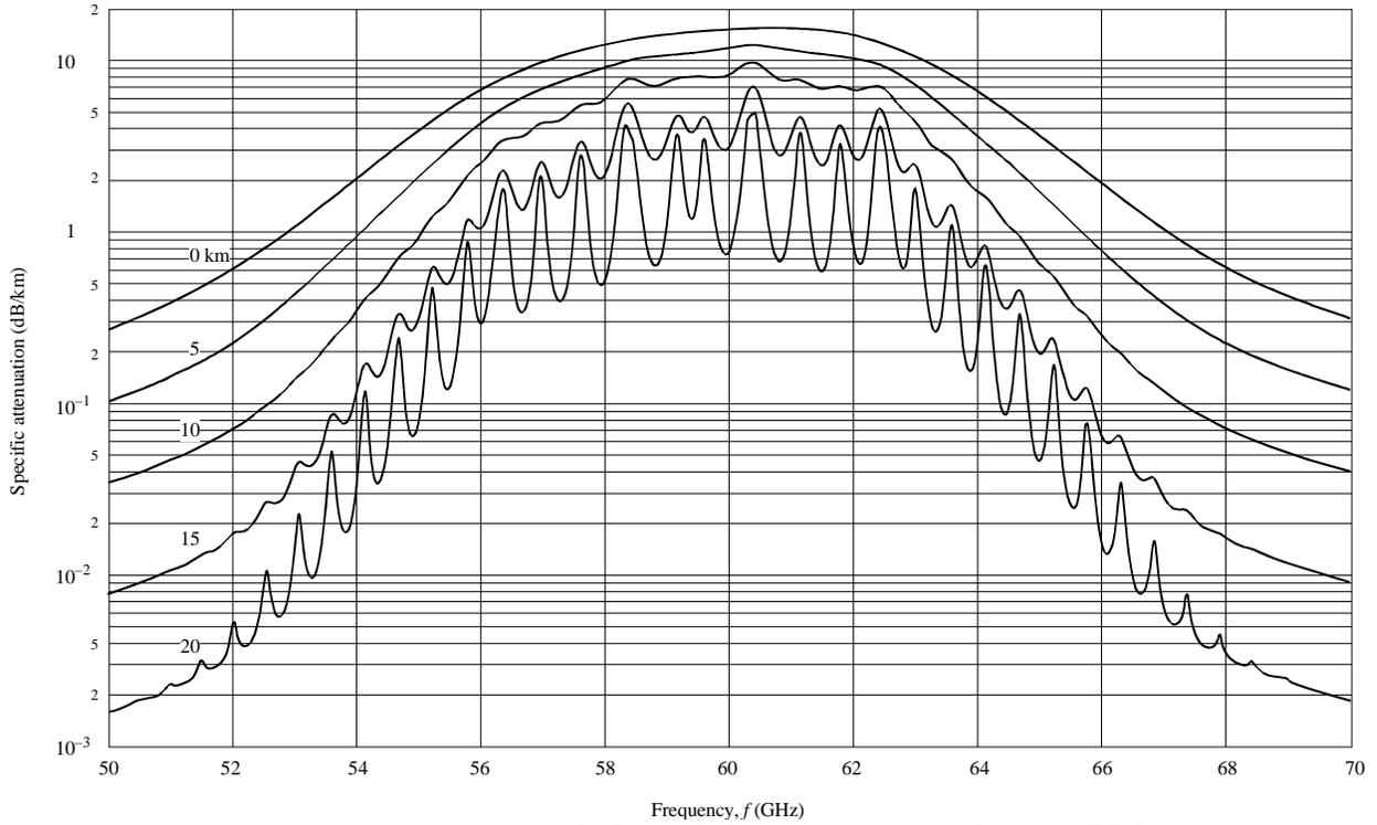
Figure A.1: Oxygen Attenuation (dB/km) – Path Land - Recommendation ITU-R P.676
