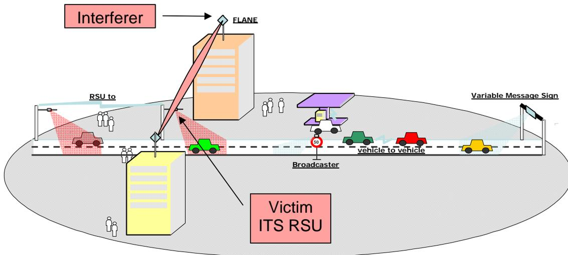
**Figure 8: Scenario 3 – ITS RSU possibly interfered with by MGWS-FLANE**
