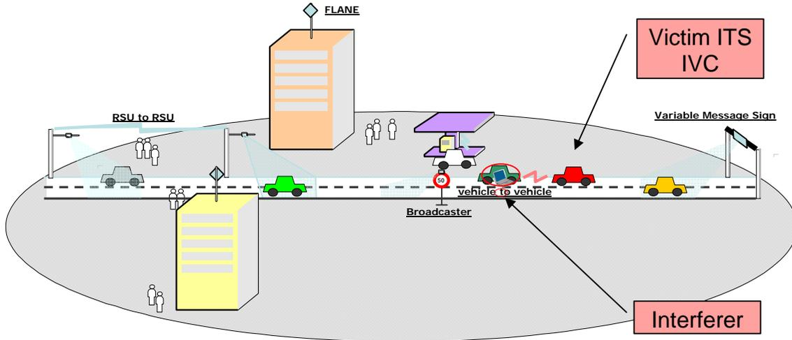
**Figure 11: Scenario 6 – ITS IVU possibly interfered with by MGWS-WLAN/WPAN located within another car**
