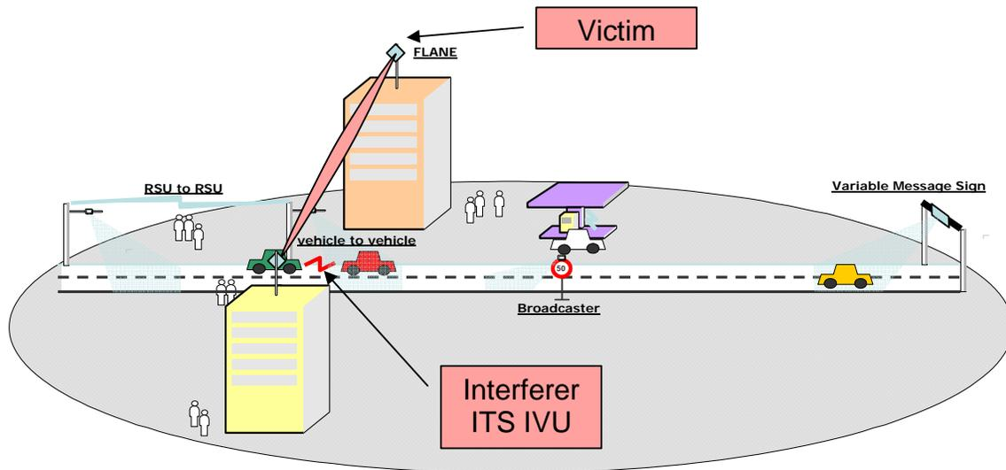
**Figure 6: Scenario 1-b – MGWS-FLANE possibly interfered with by an ITS IVU**
