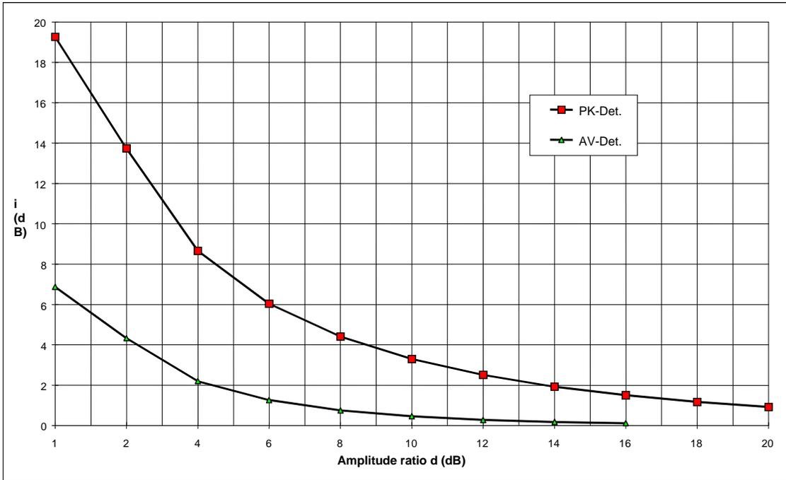
Figure A4.1: Determination of the disturbing signal amplitude by means of amplitude ratio  $d$  and correction factor  $i$
