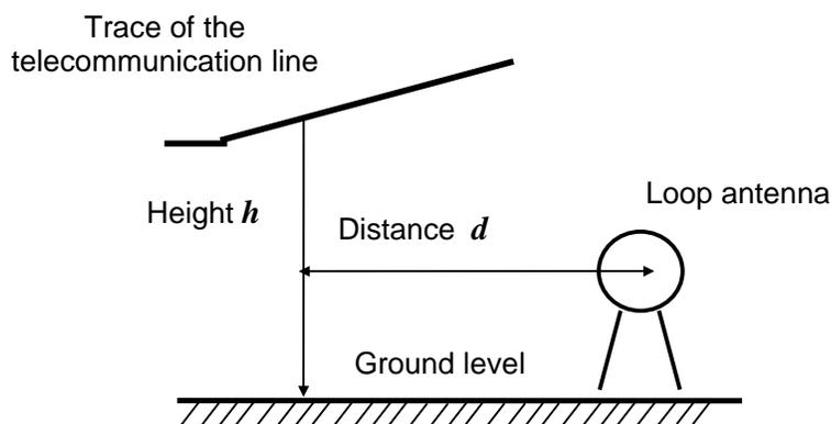
**Figure 1: Drawing the measuring distance  $d$  from the vertical projection of the trace of the telecommunication line to ground level**
