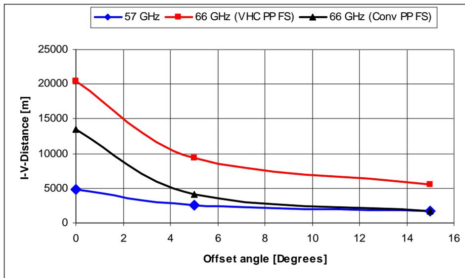
**Figure 19 : Required separation distances for scenario 5 PP FS (VHC and Conv.) Tx main beam into FLANE Rx as a function of separation angle between the links (see Figure 14 for comparison).**
