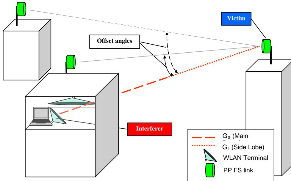
**Figure 9: Scenario 4: WLAN to PP FS Rx**
