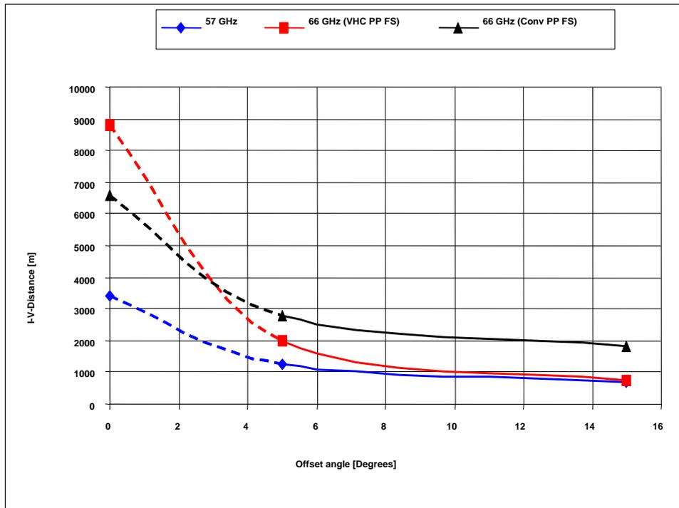
**Figure 10: Required separation distances for Scenario 1: FLANE Tx main beam to PP FS Rx as a function of offset angle between the links**
