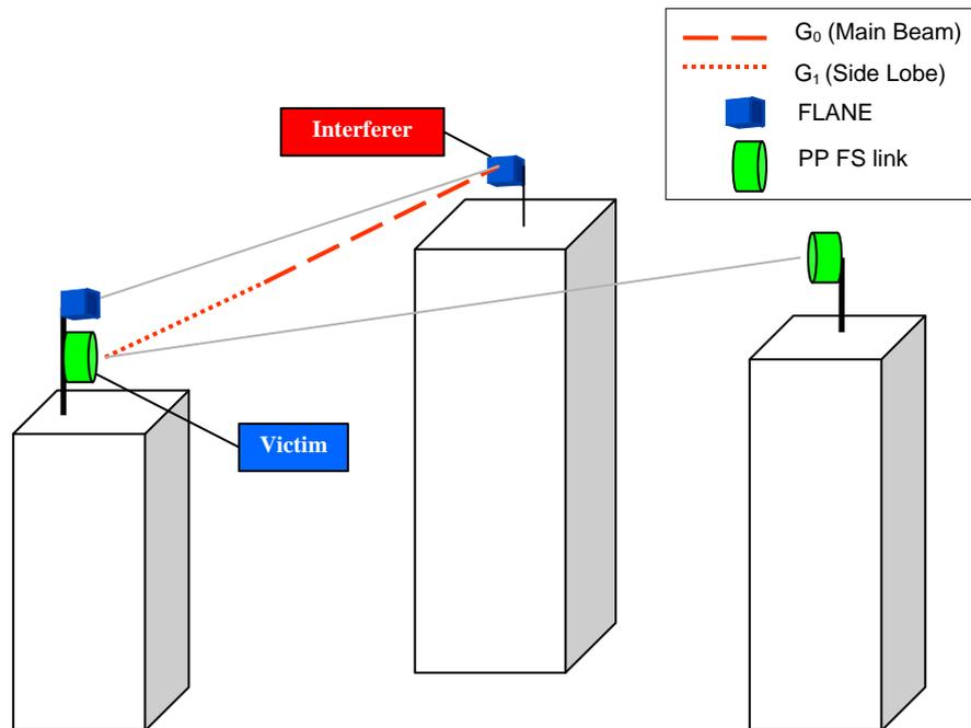
**Figure 6: Scenario 1: FLANE Tx main beam to PP FS Rx side lobes**
