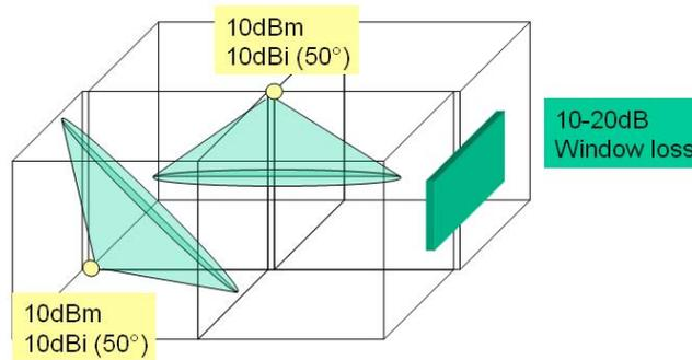
**Figure 1: Illustration of indoor WLAN deployment**
