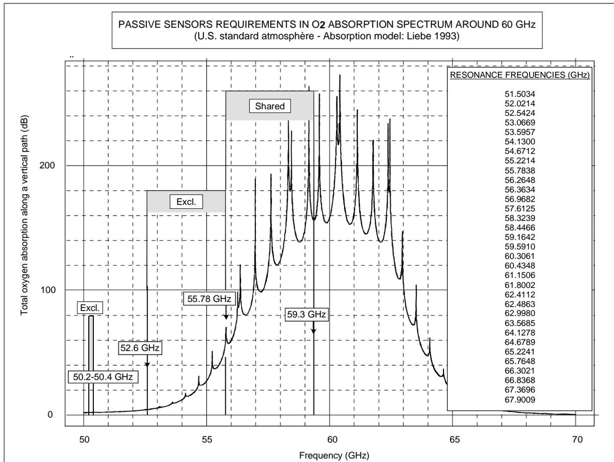
**Figure 17: Frequencies for passive sensors in oxygen absorption spectrum**
