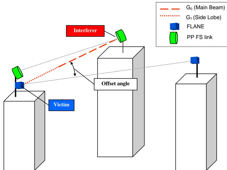
**Figure 13: Scenario 5: PP FS Tx main beam into FLANE Rx side lobes**
