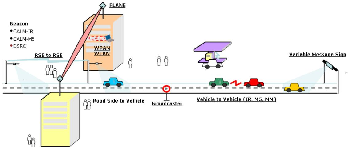
Figure 5: Example of ITS system deployment scenario, with FS links used in ITS backbone (RSE to RSE)
