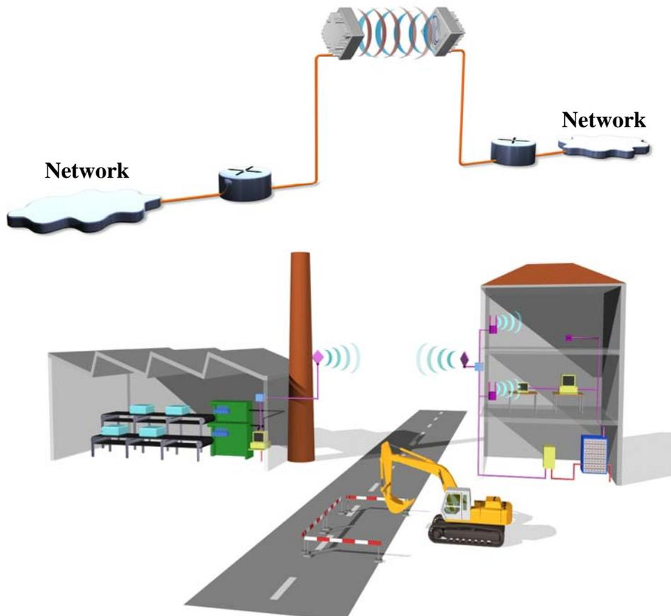
**Figure 3: Illustration of outdoor FLANE deployment**
