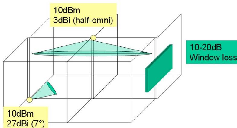
**Figure 2: Illustration of indoor WPAN deployment**
