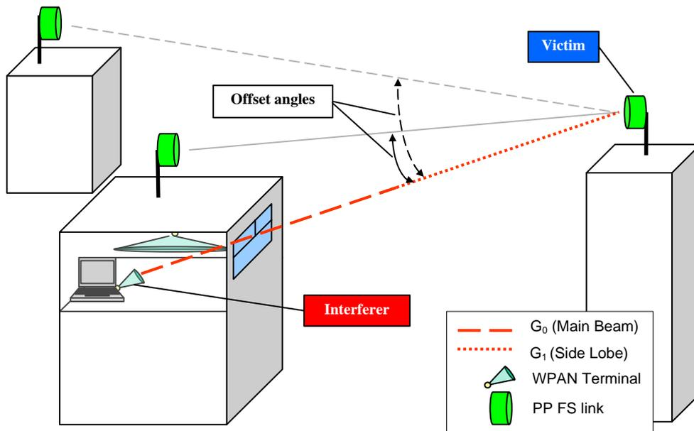
**Figure 8: Scenario 3: WPAN (note directional WPAN antenna) to PP FS Rx**
